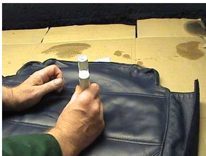
Photo 3 Checking damage with x40 microscope
